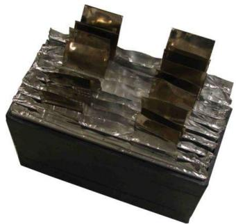
A lithium-ion polymer battery pack—with cells—is surrounded by AllCell's Phase Change Material.
